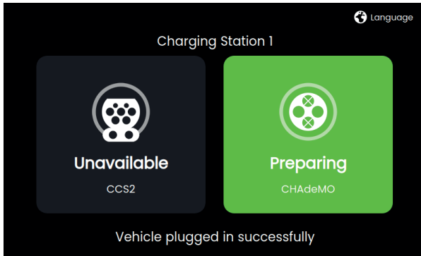
Image 14: Preparing CHAdeMO - connector plugged in
