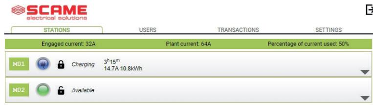
The screenshot shows the SCAME management interface. At the top left is the SCAME logo. Below it are navigation tabs: STATIONS (selected), USERS, TRANSACTIONS, and SETTINGS. A status bar displays: Engaged current: 32A, Plant current: 64A, and Percentage of current used: 50%. Below this is a table of stations:
